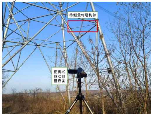
Figure 1. Measurement of the VIV in field experiments.
